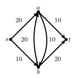
Augmenting path P = (s, b, a, t) with bottleneck capacity 10.
