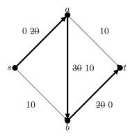
**Note:** when pushing flow, we can undo flow already pushed.
